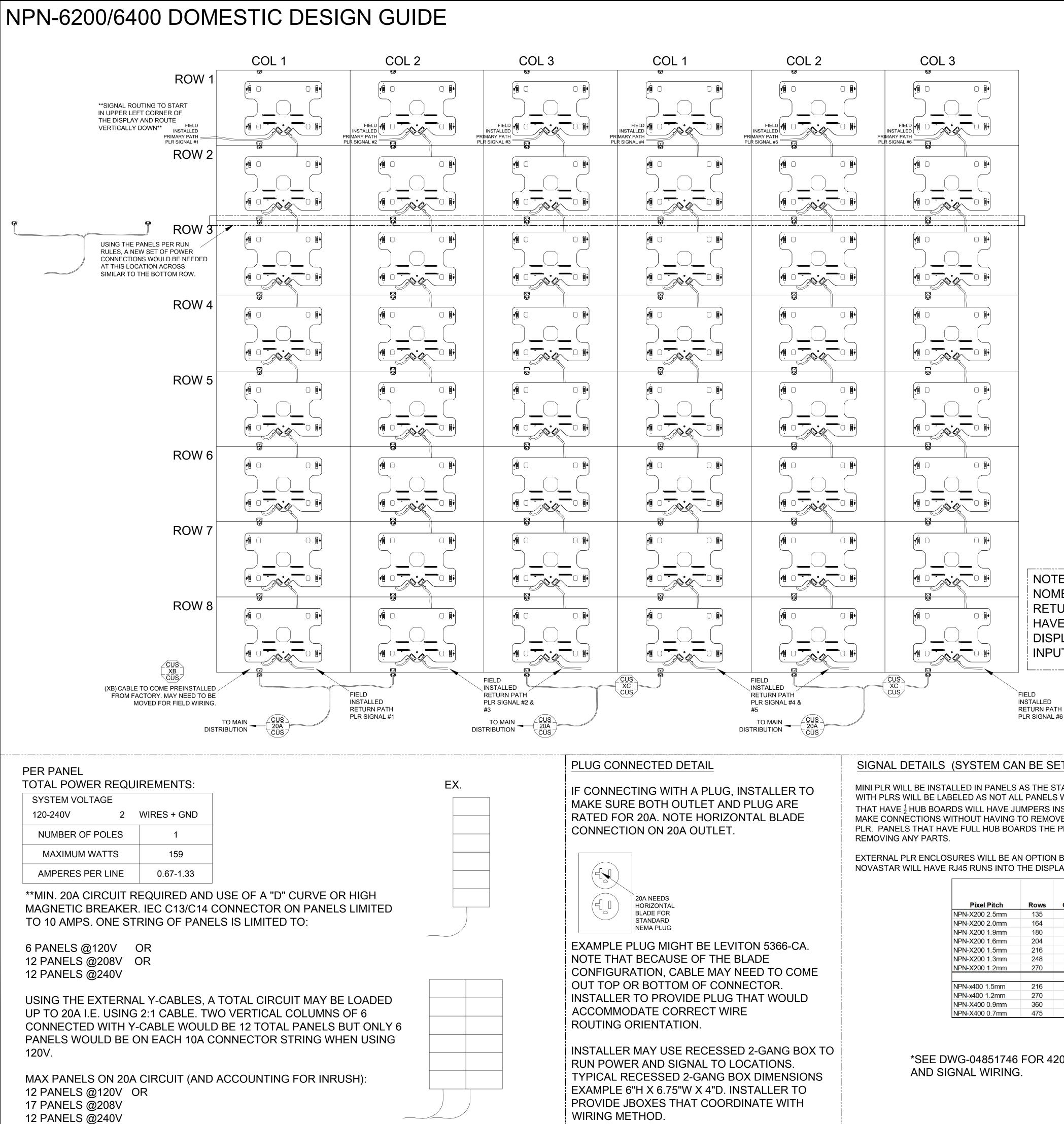
NOTE: A DISPLAY WITH A "-SR" NOMENCLATURE WILL NOT USE A **RETURN PATH TO A1 AND WILL ONLY** HAVE THE INPUT PATH TO A2. A DISPLAY WITH "-MR" WILL USE A2 AS AN INPUT AND A1 AS A RETURN AS SHOWN.
